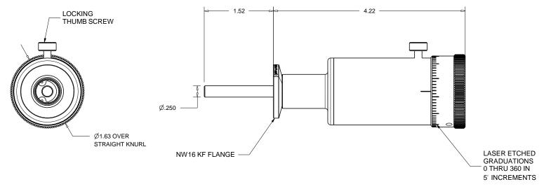
Related Flange Hardware NW16KF ISO Flange P/N 202200, Centering Ring - Stainless / Viton Hinged Clamp - Aluminum P/N 202205,
